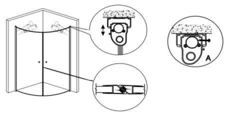
4. Install the side and the bottoM waterproof bar. Install the handle. Glue the two side by the Neutral silicone sealant
